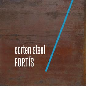
Corten Steel (CS) is a weathering steel that forms a stabilizing rust finish. This material is a corrosion resistant steel that develops an outer layer patina of rust when exposed to the environment. This process will begin here at Ultralights so that you will receive the fixture similar to its appearance in the product photography.
